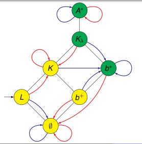
a b  $L = a^{+}b^{+}$   $K = a^{-1}L = a^{*}b^{+} = L \cup b^{+}$   $K_{\lambda} = K \cup b^{*} = K + \lambda$
